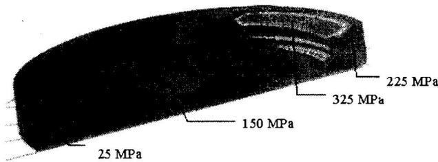
Figure 6: Von Mises stresses in pot, geometry modified by increasing the base thickness as well as the ring thickness.
