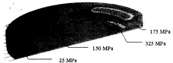
Figure 7: Von Mises stresses in pot; geometry modified by increasing the ring thickness only.
