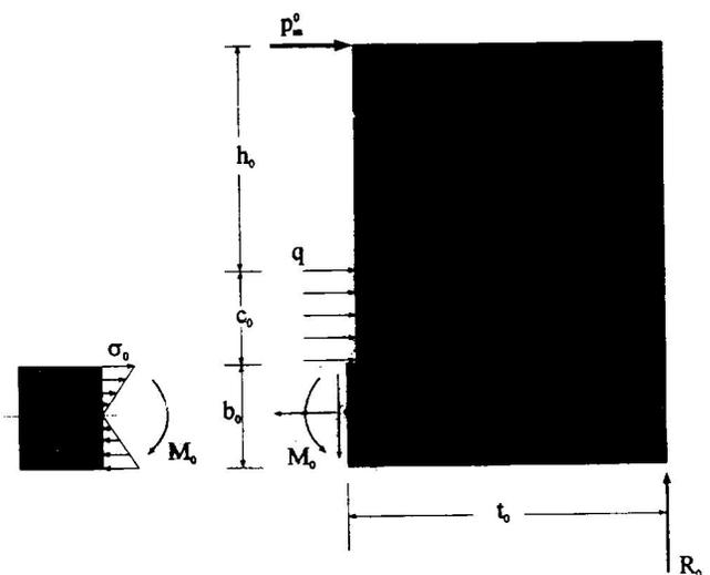
Figure 5: Two dimensional idealisation of the torsional response of pot-ring.
