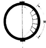
Figure 2: Distribution of seismic lateral forces on the pot
