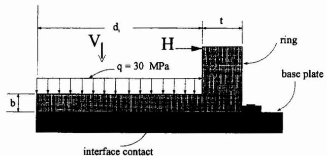
Figure 1: Cross-sectional view of a pot
